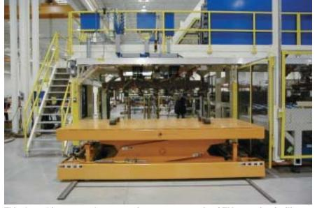
This destacking cart undergoes testing at an automotive OEM stamping facility. Note the suction-cup array located above the cart. In operation, the cart, loaded with blanks, moves into the line, and the cups grab single blanks from the stack and feed the press automatically. If desired, the empty cart can be rolled back out and another preloaded cart rolled in, ensuring continuous blank supply.
