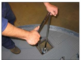
Figure 4 Example of a leveling leg being manually adjusted from the top of the lifting platform via a special access cover.
