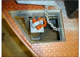
Figure  $\overline{5}$  One of four lifting shackles accessible through the lift platform.
