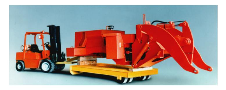
The Portavator converts a forklift into a powerful and efficient in-plant materials handling system capable of moving heavy loads using a light-to-medium duty forklift, and can be custom engineered and designed for any facility.
