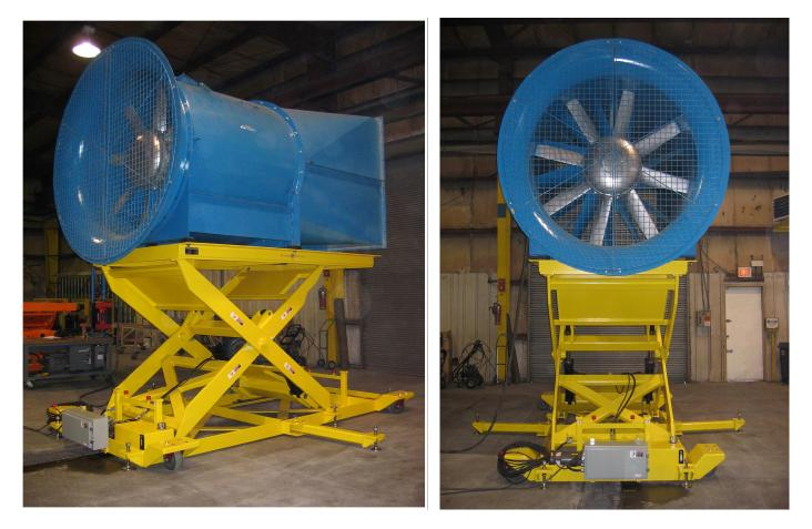
andling Specialty custom engineered and manufactured a series of portable but highly stable lift tables that supported large fans in an automotive test facility. The Factory Acceptance Test (FAT) was conducted at Handling Specialty's facilities, using the customer's actual equipment.
