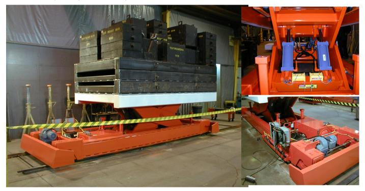
andling Specialty reached a new weight capacity limit for its automated destacking scissor-lift solutions with this project. Two hydraulic destacking lifts were engineered-to-order, each with a 60,000 lb. capacity. The lifts, built to automotive specifications, will be used for precise and controlled destacking and transferring of steel sheeting.
