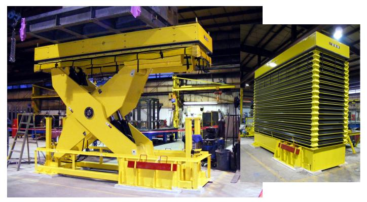
An Ohio-based gas compressor manufacturer engaged Handling Specialty to design and manufacture a high capacity, hydraulic lift to be used during the painting process. Because some of their compressors have centers of gravity outside of the lift envelope, Handling Specialty engineered a custom solution specifically for this application. In addition to the offset loads, the underside of the compressors needed to be fully accessible for painting.
