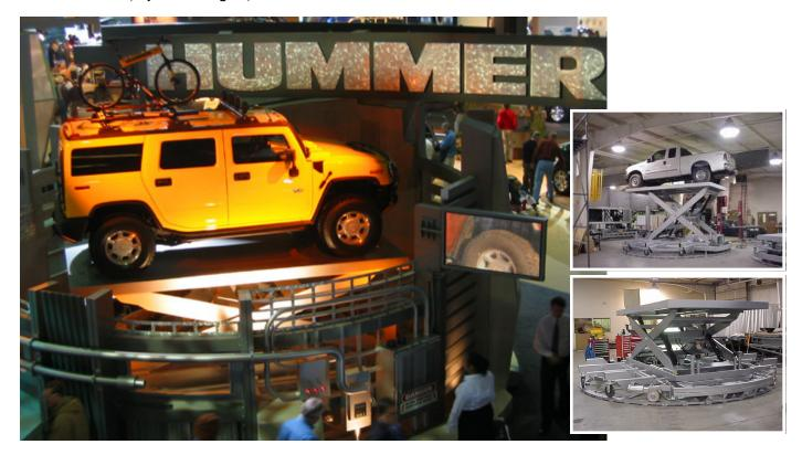
Largely based on Handling Specialty's reputation in the entertainment industry, Handling Specialty was requested to design and manufacture two lifts to be mounted onto rotators to launch the new Hummer H2 during the major US auto shows. The lifts could be programmed to automatically perform specific "moves" that were choreographed to lights, music and smoke effects during the show. The lifts could also be operated independently by handheld pendant.
