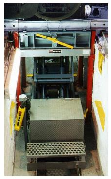
andling Specialty was approached by a mining company to engineer and manufacture a heavy duty, durable wheelset change-out system for railcars used in mining operations. The lift was manufactured to last in the extreme conditions that exist in mining facilities in northern Canada.
