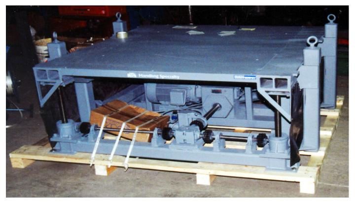
andling Specialty custom designed and manufactured a mechanically-actuated shim table for a Canadian locomotive maintenance facility. The table is used in the shimming process which adjusts wheel diameter differentials.
