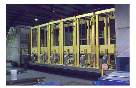
andling Specialty custom engineered and manufactured six pit mounted assembly stations for a major airplane engine manufacturer. The customer required that the lifts could not be visible above floor level at any time and had to provide smooth, synchronized, level lifting through the entire range of travel to prevent jarring of the engine.
