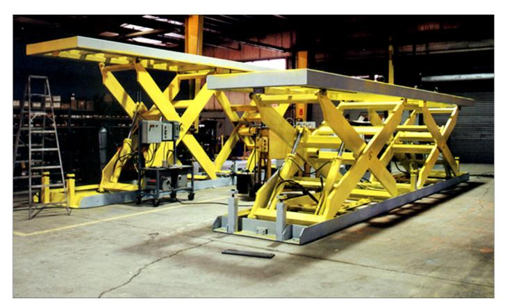
andling Specialty custom designed and manufactured two direct thrust hydraulic stage lifts to lift and hold performers at a theme park. The pit-mounted lifts are operated in unison or independently and are situated on either side of an arc-shaped stage area. Two sets of scissors were used on each lift to reduce the differential deflection of the long platform due to the movements of show personnel during performances.
