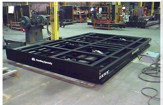
The University of Cincinnati's Music Conservatory contacted Handling Specialty to custom design and manufacture a hydraulic scissor lift to convey props/set pieces to the conservatory's upper level, while also being used as a 10,000 lb capacity rollover access to the stage in the lowered position. When not in use, this pit-mounted lift remains in the fully raised position.
