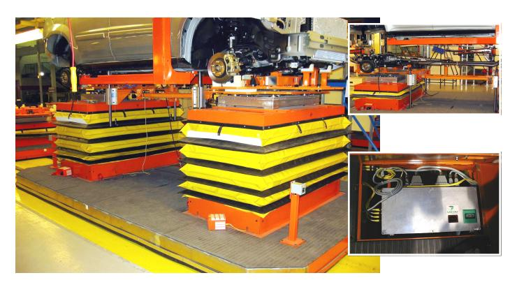
andling Specialty engineered and manufactured custom towveyor carts that move both horizontally (by towline) and vertically (with two electromechanical lifts) to meet the ergonomic and assembly needs of an automotive production line. The front lift is used to hoist the front axle and engine assembly into the vehicle body while the back lift inserts the rear axle. Synchronous lifting is essential since the front and rear modules are joined by a drive shaft.
