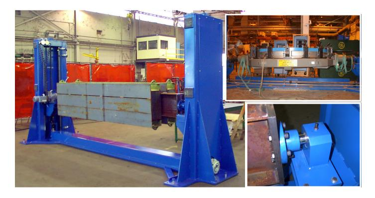
andling Specialty engineered and manufactured a custom two post rotating mast lift for an international power company's (GE) power generation facility for turbine equipment inspection.
