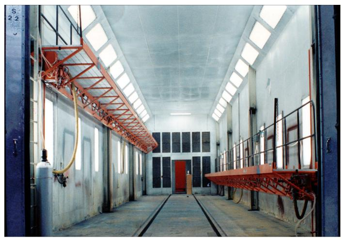
andling Specialty can custom engineer and manufacture wall mounted lift platforms the railcar painting and stenciling process. Vertical travel, capacity, and overall platform size can all be varied to suit the exact specifications of any paint facility. Lifts can also be engineered and manufactured for Class 1 Div. 1 specifications (explosion proof).
