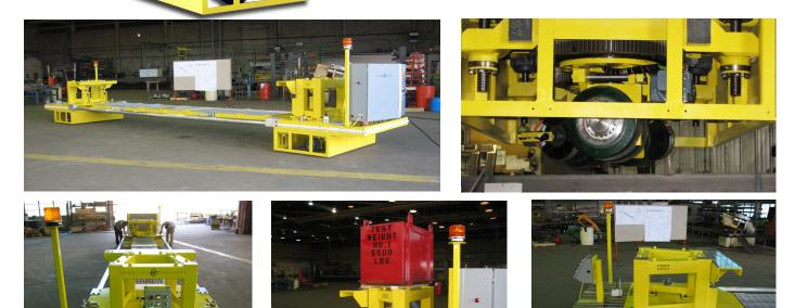
andling Specialty custom engineered and manufactured a motorized transport cart to assemble and test classified equipment for a major US defence company. Length of the component varies between 24 to 30 feet and weighs upward of 3,000 lbs.
