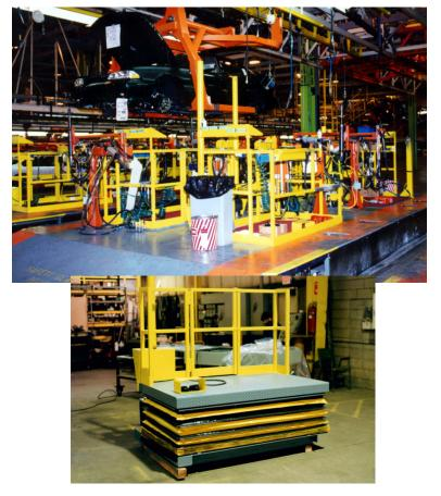
One of the original "Big Three" North American automakers approached Handling Specialty because it needed an ergonomic, clean and safe employee lift for its drivetrain and chassis marriage line. Because of the application, a precise and smooth motion was essential.
