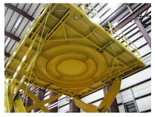
andling Specialty custom engineered and manufactured a vertical assembly platform to be used during the assembly process of large energy turbines. The lift rises 21 feet at full extension and its lowered height is less than eight feet. A scissor lift was chosen (over a four post lift) to take advantage of an existing pit in the facility.
