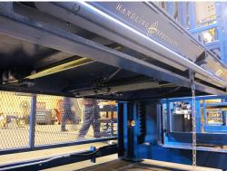
andling Specialty designed and manufactured six (6) personnel lifts for an international engine manufacturer in the USA. The lifts will be operated in pairs and will allow technicians to position themselves at different elevations throughout the assembly process of large engines (such as locomotive engines).
