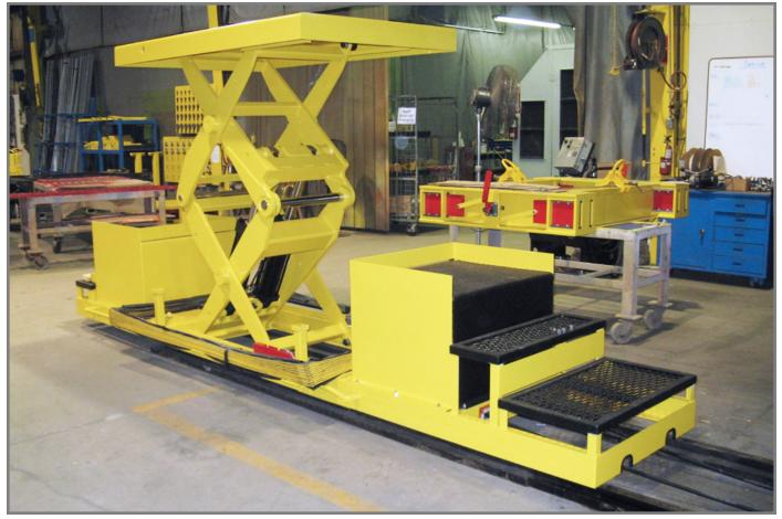
andling Specialty was approached by a mining company to engineer and manufacture a heavy duty, durable wheelset change-out system for railcars used in mining operations. The lift was manufactured to last in the extreme conditions that exist in mining facilities in northern Canada.
