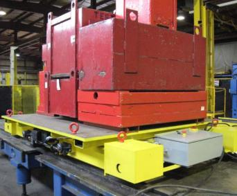
andling Specialty was approached by a previous customer, Siemens, to custom engineer and manufacture a portable lift capable of moving 35,000 lb locomotive transformers in a locomotive assembly facility. The lift, which moves the transformer underneath the locomotive, traverses along the track and can move up or down 2" and cross traverse 2" in each direction to aid in the installation of the transformer.
