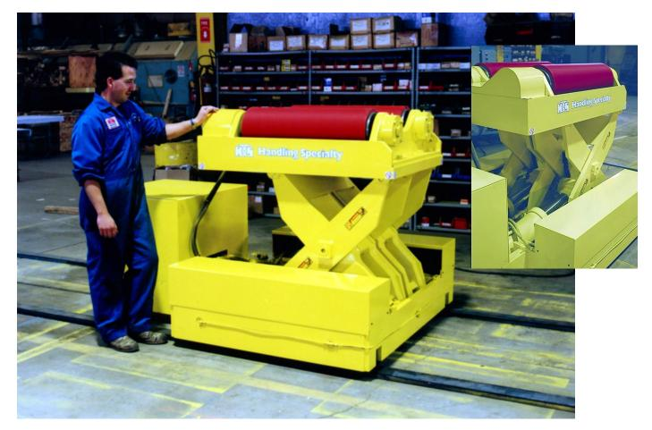
andling Specialty was presented with a material handling challenge by steel giant Allegheny Ludlum to move steel coils through an existing narrow pit system. Fitting within 3/4" of the pit walls, the 50,000 lb. capacity lift measures only 64" wide and 84" long.
