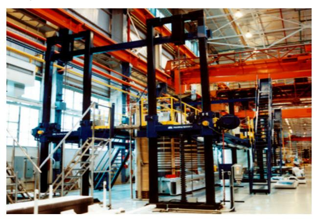
andling Specialty custom engineered and manufactured an assembly work platform that helped improve workers' efficiency and safety. Incorporated in the design are platforms that extend 60" in and out enabling employees to reach an optimal work position.
