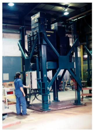
A solution engineered to help assemble 20 foot electrical transformers gave birth to one of Handling Specialty's multi-industry multi-use heavy duty robust four post pit or floor mounted Cargovator. When transformers began being assembled vertically, companies required a way to safely hold and raise and lower the equipment as it was being worked on.
