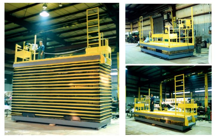
andling Specialty's self propelling 4,000 lb capacity personnel platforms were used to help Thrall Car Manufacturing manufacture railway cars used to transport automobiles during the company's height of production. The lift carried workers vertically and horizontally alongside the rail car allowing them to work at any elevation, while travelling along 200' of track.
