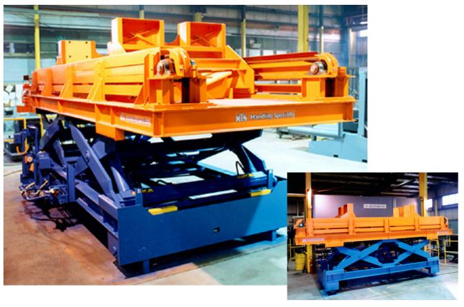
An international steel company in the US required two custom designed rugged and durable steel transfer cars to handle large bundles of accumulating wire rod and transfer it between process lines.
