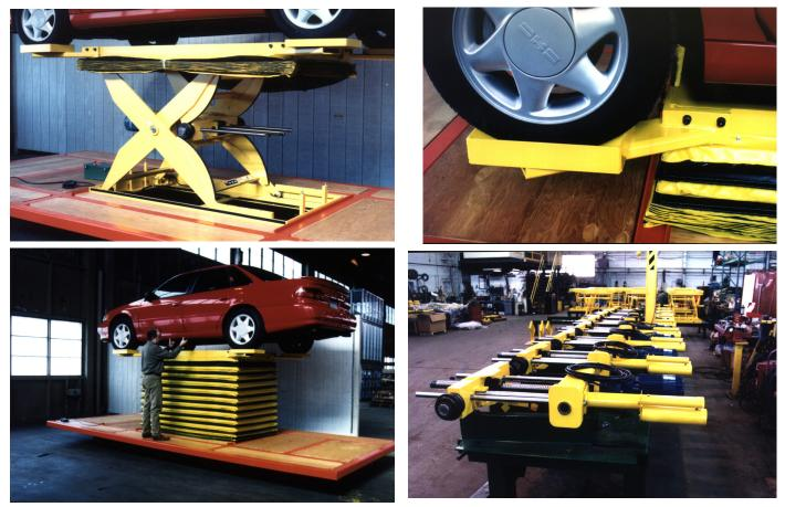
andling Specialty helped pioneer the modern automotive assembly line back in the early 80s with the development of ergonomic and efficient skillet lifts for the North American auto industry. The lift allows the vehicle to to be raised and lowered by foot controls. As the line moves, employees adjust each vehicle's height to their own ergonomic requirements.
