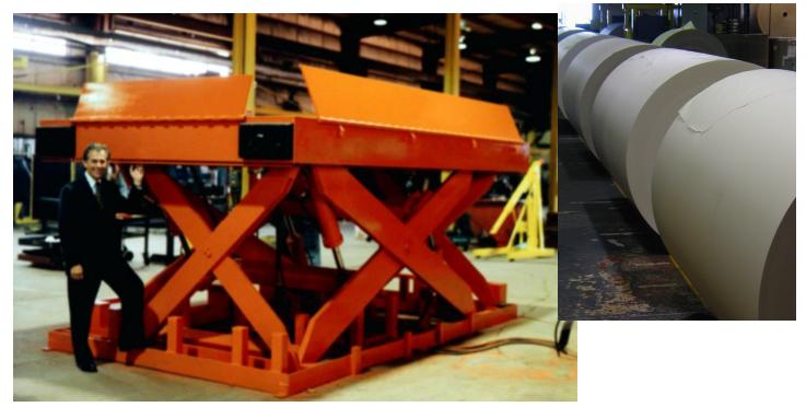
F or the Houston Chronicle, Handling Specialty custom engineered and manufactured a 20,000 lb. capacity lift for the unloading of 5,000 lb. paper rolls. The high demand for newsprint at the newspaper required the lift to endure heavy use. As well, Handling Specialty engineers had to incorporate into the lift support for a large side load that was created as a fork truck drove onto the lift from the side. In order to address this, crossstabilizing scissors were employed to provide extra strength.
