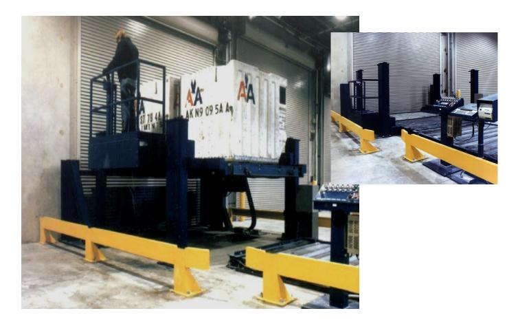
A four post mechanically actuated Cargovator was the ideal solution for air-cargo logistics at American Airlines Ain Dallas, Texas.
