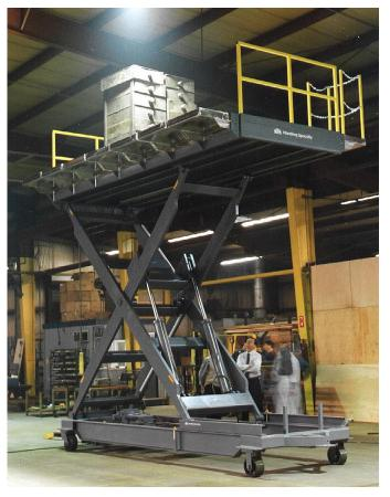
andling Specialty custom designed and manufactured an accurate and precise lift to replace gimbles for a nuclear energy provider in Canada. Located on the underside of a crane inside the nuclear facility, a gimble is used to replace fuel rods in the reactor.
