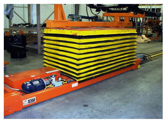
andling Specialty played a significant part in the development of the modern assembly line used in automotive assembly plants today. This lift is a prototype that was developed for a Big Three automaker in the 80s as efficiency and ergonomics became an integral part of the auto assembly process. These self-propelled lifts were custom engineered and manufactured by Handling Specialty and were used in a simulated auto assembly plant environment to develop new processes and train workers.
