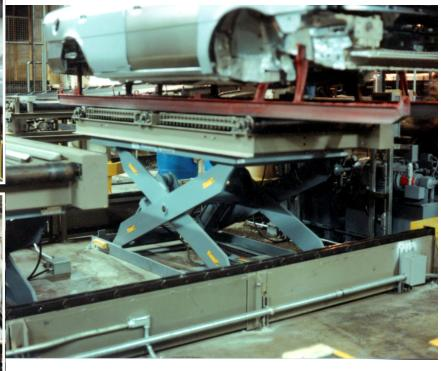
andling Specialty solved a material handling challenge in a Canadian auto plant by custom engineering and manufacturing a high cycle, robust and durable lift system that transferred car bodies atop steel skids between two sets of conveyors set on different levels.
