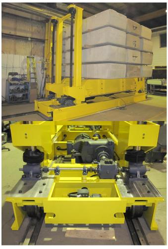
A large railroad maintenance facility in the United States required a 50-ton drop table to facilitate the change-out of traction motors on its locomotives. Handling Specialty custom engineered and designed a 50 ton drop table that is based on an original heavy duty Whiting Corporation design.
