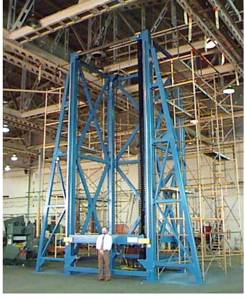
A major aerospace and defence integration firm approached Handling Specialty to custom engineer and manufacture an automated ultrasonic inspection system to inspect the exterior surface of a rocket shell using a robot. The lifts/robotic units work in tandem: one robot repeatedly raises and lowers inside the rocket shell on the scissor lift while the other matches this movement on the outside via the four-post lift.
