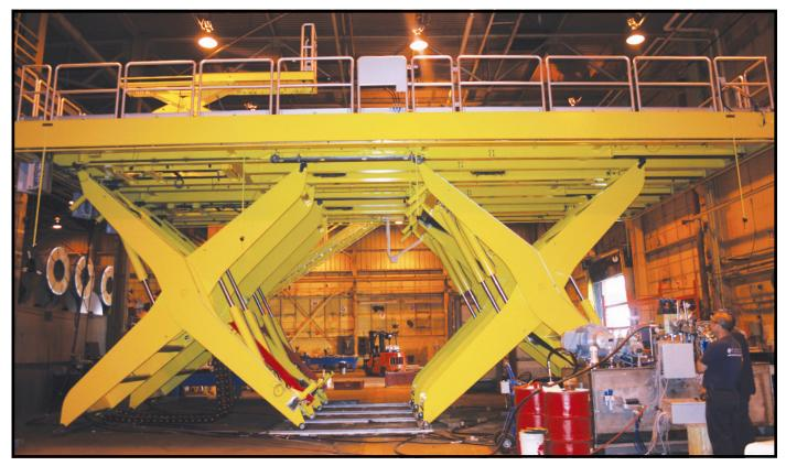
andling Specialty was approached by an internationally-recognized aerospace company (and previous customer) to design and manufacture a heavy duty, long-lasting, explosion proof material handling lift for use in a jet engine test cell. The lift is being used to load new jet engines into a test cell for testing and to safely and reliably move personnel and equipment around the jet engine.
