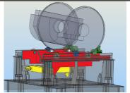
Existing wheel chocks are placed behind the TM wheels. The new sliding wheel chocks are installed on the front side of the TM wheels.
