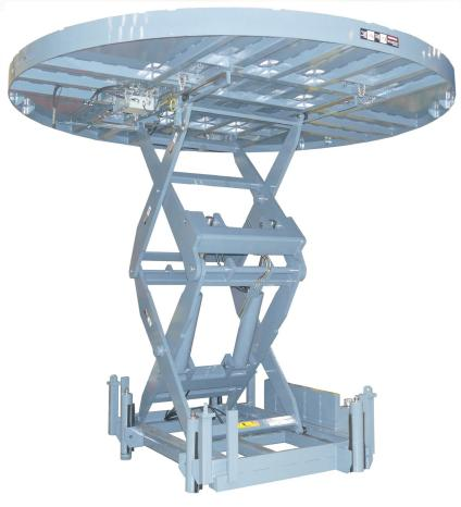
Custom ladle rebricking/relining lifts have replaced scaffolding/platforms used in the rebricking process to improve safety, reduce downtime and incre ase productivity.
