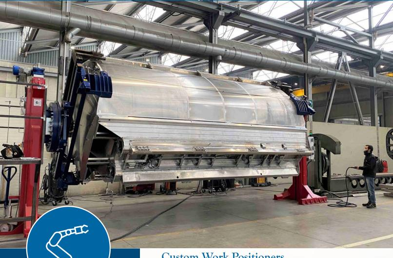
Custom work positioners are designed to provide ergonomic, full rotational access along the horizontal and vertical axis for positioning custom, heavy weldments with large offsets.
