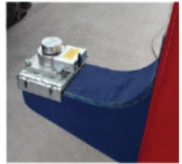
Loading cell system for weighing
